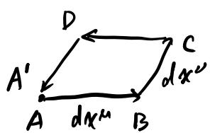
$$\begin{aligned} dV &= V_A - V_A' \\ &= [(V_C - V_D) - (V_B - V_A)] - [(V_C - V_B) - (V_D - V_A')] \\ &= \nabla_\nu dx^\nu \nabla_\mu dx^\mu V - \nabla_\mu dx^\mu \nabla_\nu dx^\nu V \\ &= dx^\mu dx^\nu [\nabla_\nu, \nabla_\mu] V \end{aligned}$$
